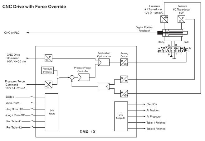
Force Feedback - Most force control applications will use two pressure transducers that output 0 to 10 VDC. #2 Transducer input cannot be
