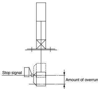
3. In order to further improve stopping accuracy, the time from the stop signal to the operation of the lock should be shortened as much as possible.
