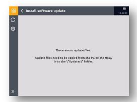
Update files for the device always have to be transferred manually from the PC to the HMG 4000 and into the folder "HMG / Updates". Multiple update files can be saved to the device at the same time.
