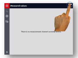
By tapping the battery/time field in the display bar, the adjacent "Status window" will open.
