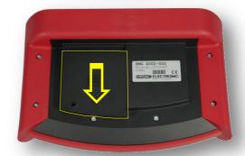
Loosen the connection plug of the battery pack.
