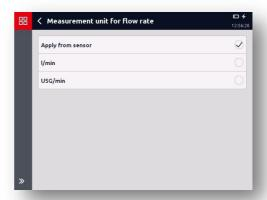
The settings in this menu always apply to all analogue measurement channels and all connected HSI sensors with automatic sensor detection!
