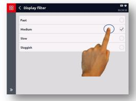
The settings for the display filter in the measured value display do not influence the measurement itself! They solely serve to settle down the display, for example, with pulsations.
