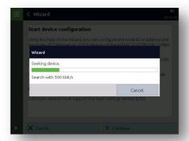
If the connected device is "found" (detected), you can change the node ID and baud rate according to the requirements.
