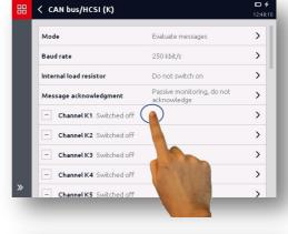
If you selected and activated a (CAN bus channel Kn), the adjacent configuration window will open.
