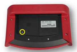
Move the battery compartment cover downward, over and past the block.
