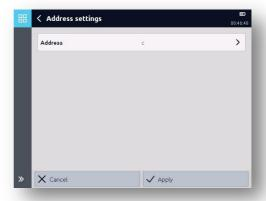
Bus addresses must be assigned when the SMART sensor is operated in a bus system. (This function is not described further here).
