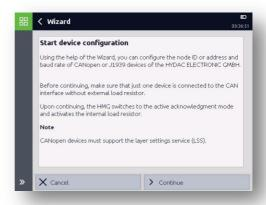
The values currently set in the device for node ID and baud rate as well as the device status and configuration do not have to be known for the search to function! All information is read out using the search function of the HMG 4000.
