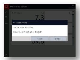
There is one exception where the null shift is automatically deleted. This happens when a sensor is connected to the channel and this sensor has a different measurement range to the one for which the null shift was set.
