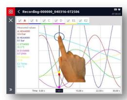
Here, too, the differential between a selected starting and end point of a particular curve section (e.g. of a pressure pulse) can be rendered and measured.
