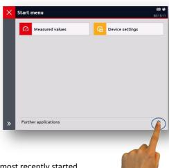
Using the button in the "Further applications" field, additional functions or applications of the device will be shown for selection:
