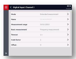
The measured value is calculated by multiplying a basic measured value with a scaling factor and then adding the offset value to this.
