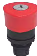
Push Key Mushroom. Manual push "In". Automatic latches "In". Turn key clockwise to release. Spring return. Key withdrawable "Out" position only. Red only.
