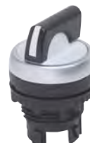
Automatic Push/Turn Mushroom. Manual push "In". Latches "In". Turn clockwise to unlatch. Spring return.
