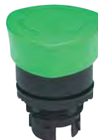
Automatic Push/Turn Mushroom. Manual push "In". Latches "In". Turn clockwise to unlatch. Spring return.
