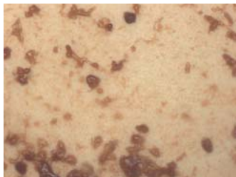
◀ Greasy/resinous residue, 500 x
