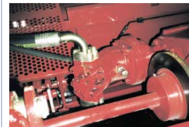
3-speed mechanical shift gearbox with fixed displacement motor A2FM
